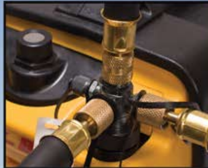
Full Flow: Use direct connections, large hoses, and no restrictions
